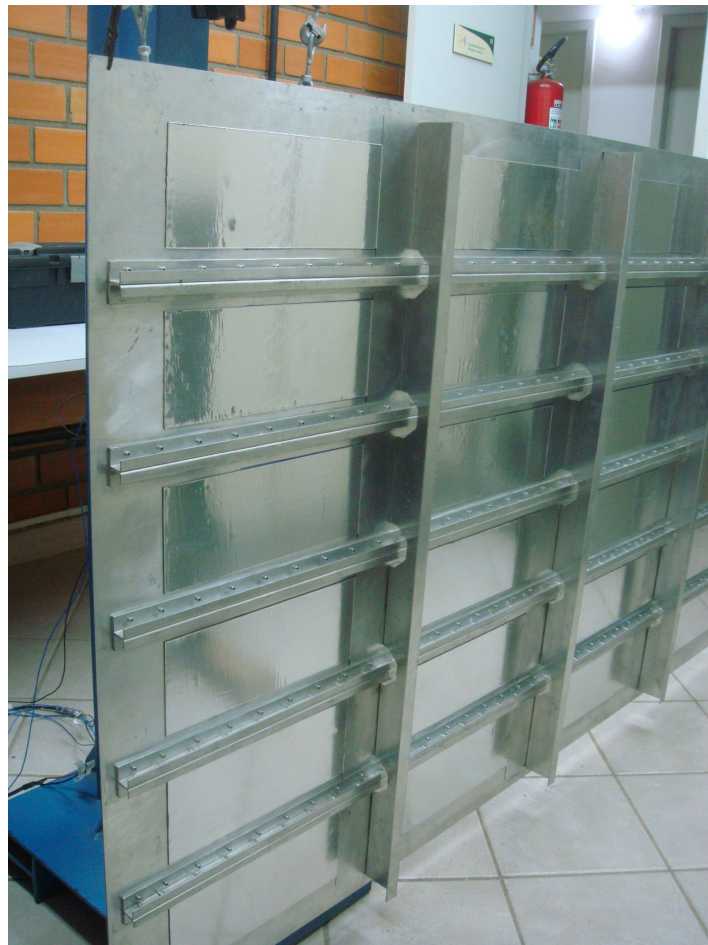
Figure 5. Fuselage panel with viscoelastic material applied in the bays.
