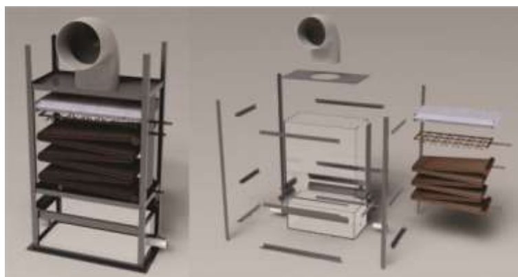
Figure 4. On the left, the virtual model of the evaporative condenser and on the right, its exploded view (Walther, 2009)
