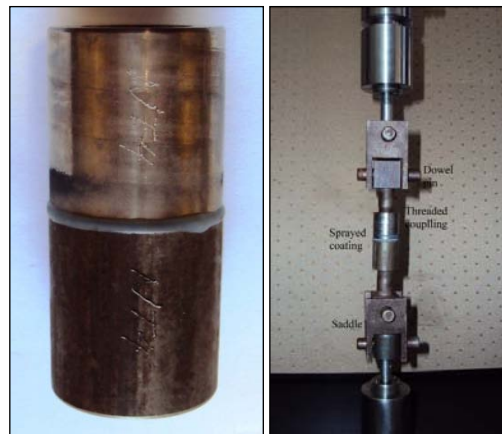
Figure 3. Image of adhesion testing.
