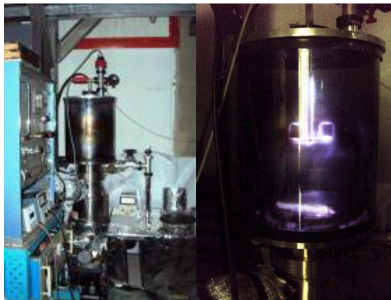
Figure 2. System vacuum heat treatment.
