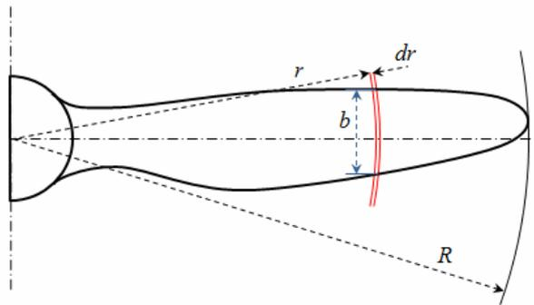
Figure 1. Infinitesimal airfoils along the blade radius
