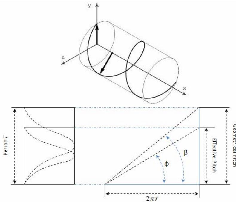
Figure 3. Path developed by an element together with corresponding geometric and effective pitch
