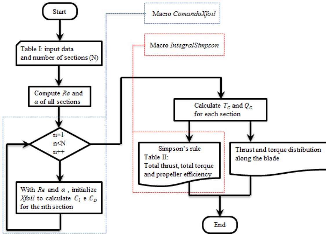
Figure 7. Complete algorithm flowchart
