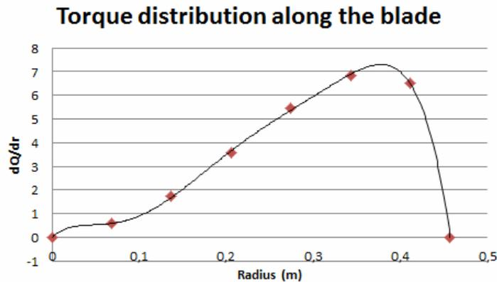
Figure 13. Torque distribution along the blade
