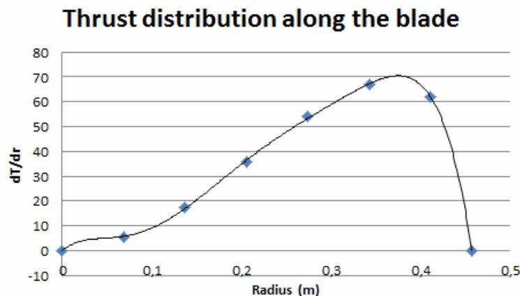
Figure 13. Thrust distribution along the blade
