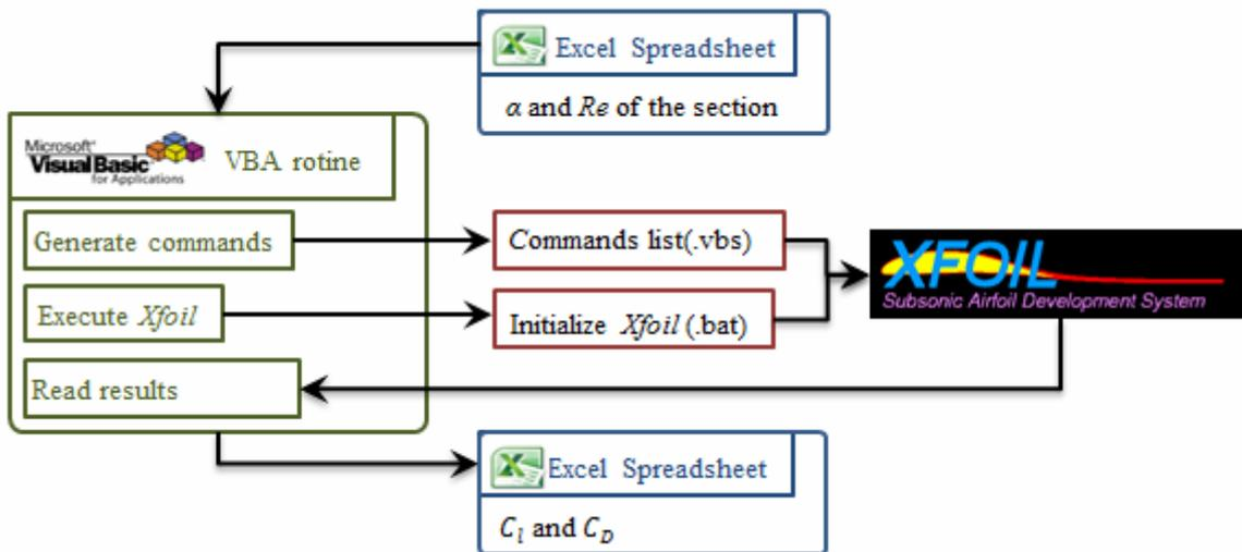
Figure 5. Method used to calculate aerodynamic coefficients
