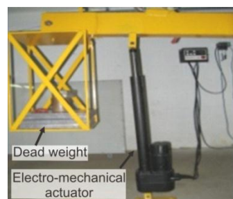
Figure 4 – Actuator connected to the lever arm in order to maintain the mean stress level in the cable within a \pm 1\% of its nominal value.
