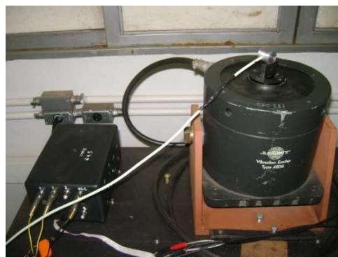
Figure 6: Mounting the accelerometer and standard block on the shaker.
