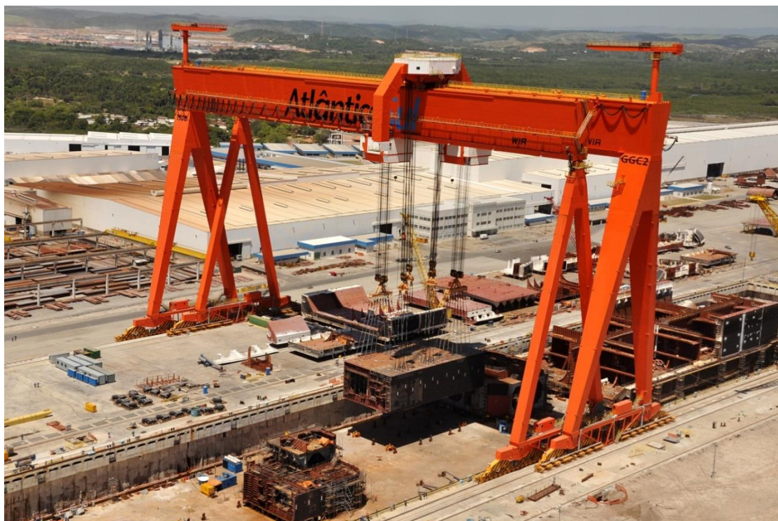
Figure 3. A 25.000 kN block for P-55 offshore platform being lifted at Atlântico Sul shipyard. Photo courtesy of Estaleiro Atlântico Sul .
