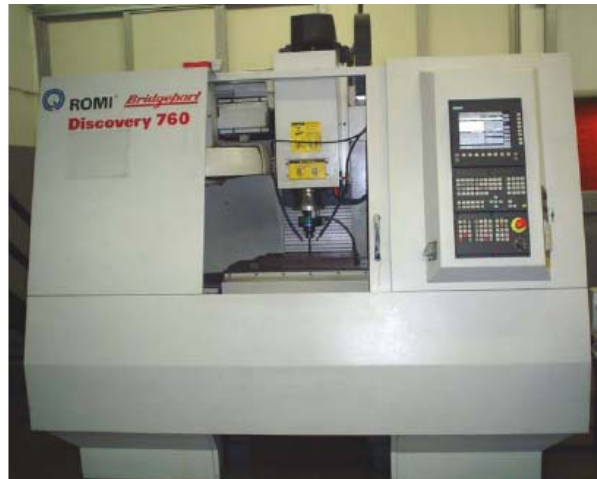
Figure 1. Vertical CNC machining center used in the drilling tests
