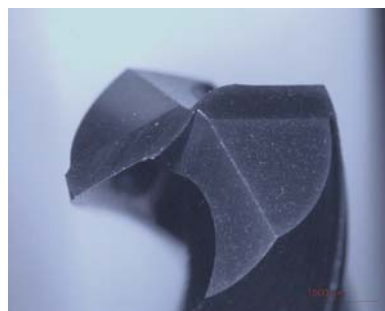
Figure 2. Geometric aspects of the TiN-TiAlN drills: chisel edge and clearance surface
