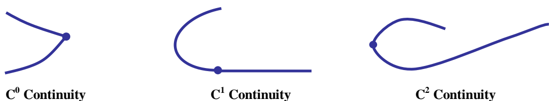
Figure 2. Curves with C^0 , C^1 and C^2 geometric continuity between their segments. (Adopted from Salomon, 2006, pp. 17).
