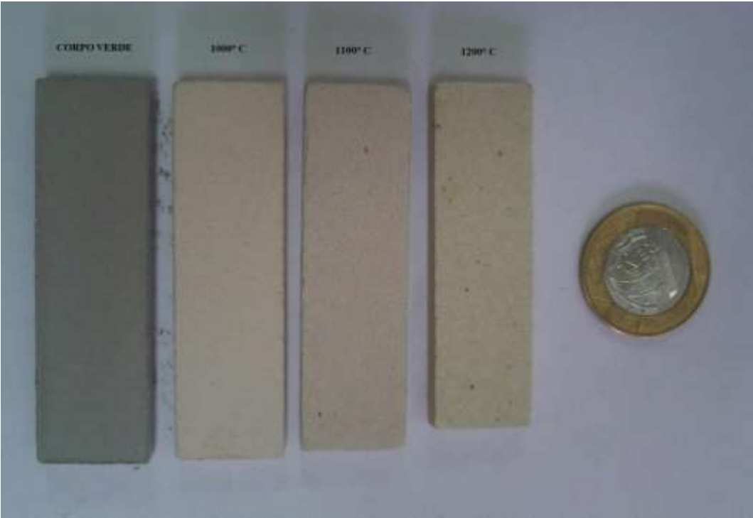
Figure 9. Photographs of samples containing Li-feldspar, before and after sintering at 1000, 1100 and 1200°C, showing coloring and retraction.
