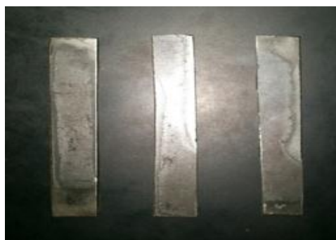
Figure 6. Samples of 1010 steel (C7*) before the impact test
