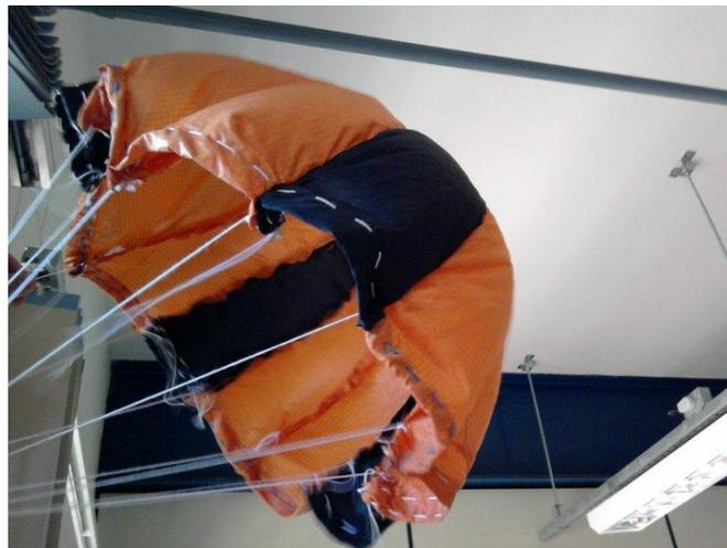
**Figure 1:** Small elliptic model parachute used in experiment.
