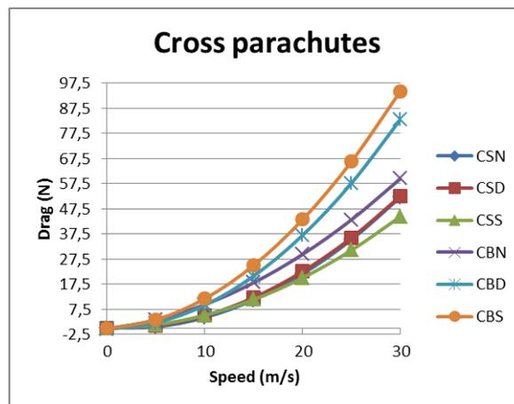
**Figure 3:** Regression plots for cross parachute configurations.
