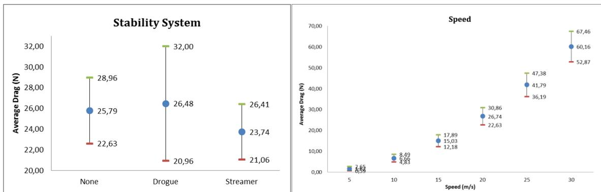
**Figure 6:** Parachute stability system and speed influences.
