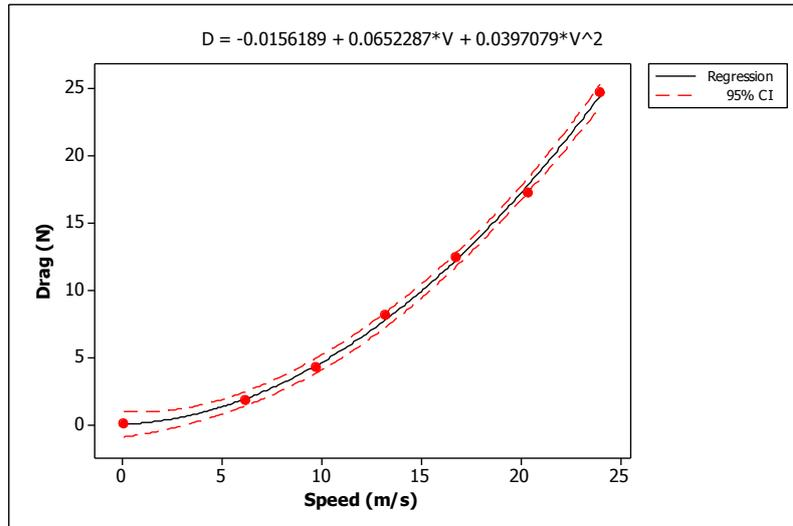
**Figure 2:** RSD test non-linear regression plot with confidence interval.
