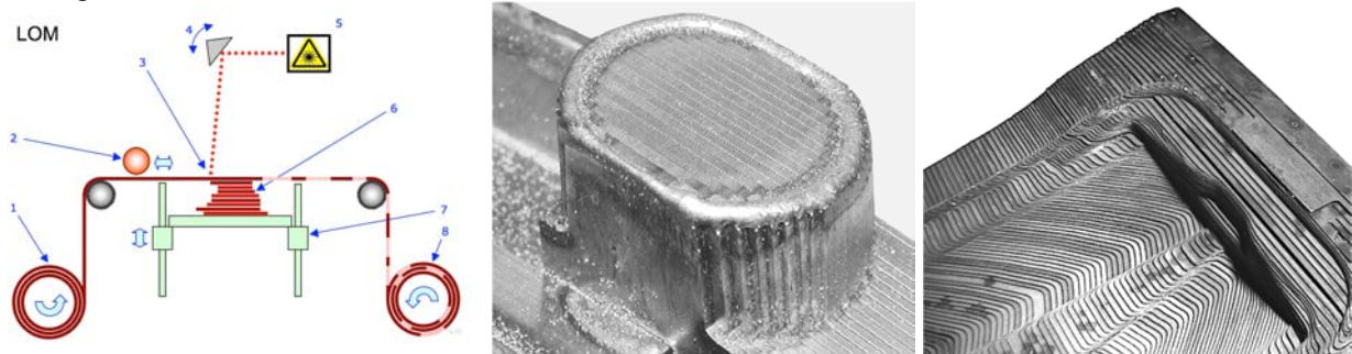
Figure 3. Cutting Process and LOM used for rapid tooling in die manufacturing.
