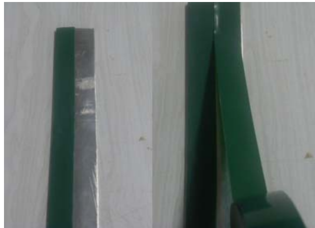
Figure 1. Fabricating the aluminum beam with double side tape.
