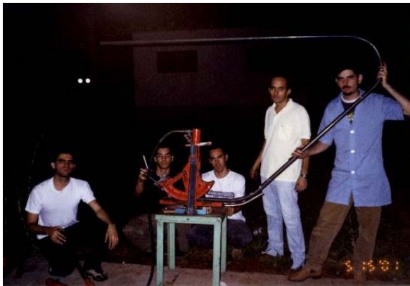
Figure 3. Construction of the vehicle. On the left students curving a tube for the structure, on the right the mounted structure
