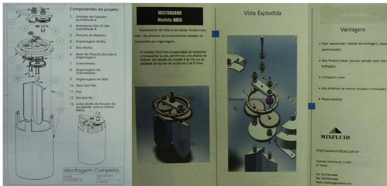
Figure 7. Planetary reducer projected by a group of student.
