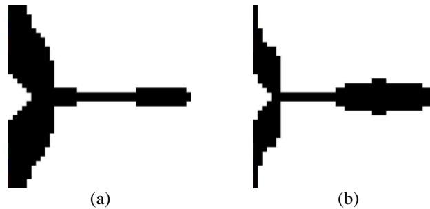
Figure 5 – Interpreted topologies: (a) Static optimization; (b) Dynamic optimization.
