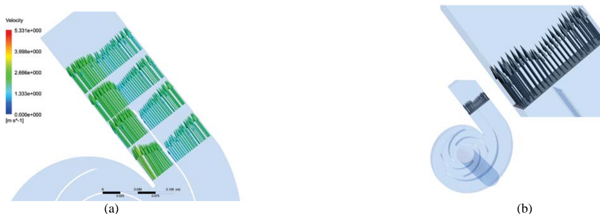
Figure 10. (a) Velocity field at the cross section of volute throat; (b) Velocity components of the plane parallel to the volute outtake.
