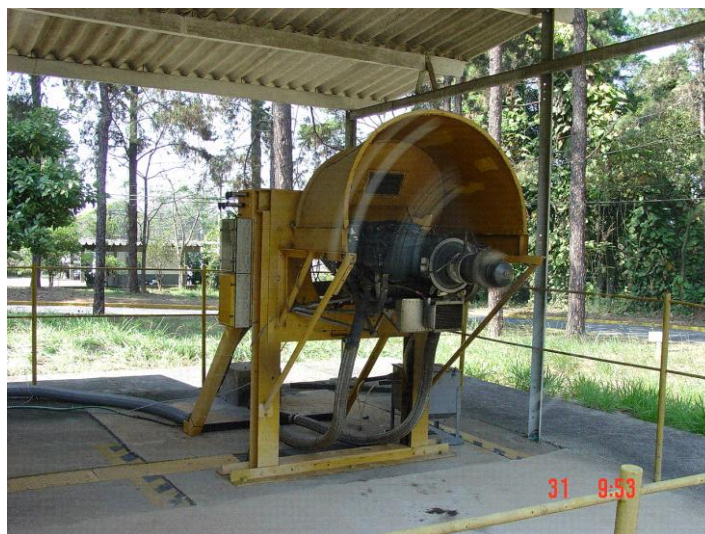
Figure 1 - Lycoming IO-540 engine mounted in test bench
