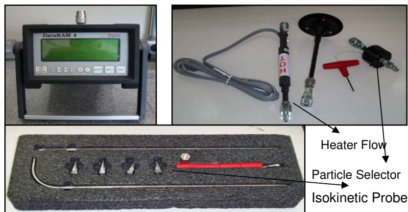
Figura 4 – Illustrative pictures of DataRAM 4 and peripherals
