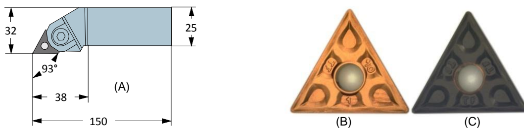
Figure 4. Tool geometry assembled on tool holder (A) (dimensions in millimeters), IC9250 insert (B), and IC8250 insert (C).
