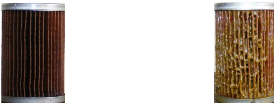
Figure 5. (a) left, fuel filter after 50h of diesel operation. (b) right, fuel filter after 50h of B100 operation.
