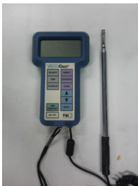
Figure 5. Hot wire anemometer
