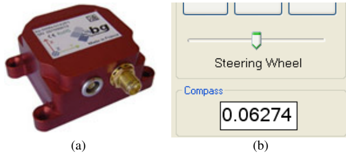
Figure 6. IMU SBG IG-500 sensor. (a) Sensor image. (b) Virtual compass representation
