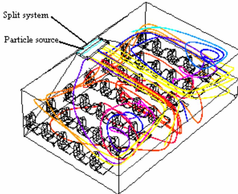
Figure 7. Particle trajectories ( $1\mu\text{m}$ ) for particles released from the outlet of the equipment
