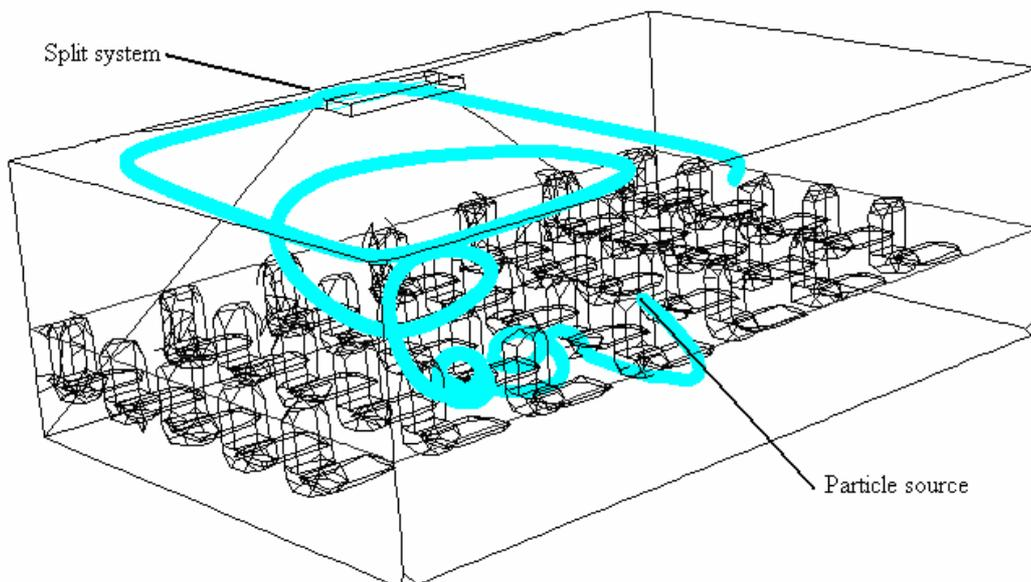
Figure 4. Particle trajectory (1  $\mu\text{m}$ ).
