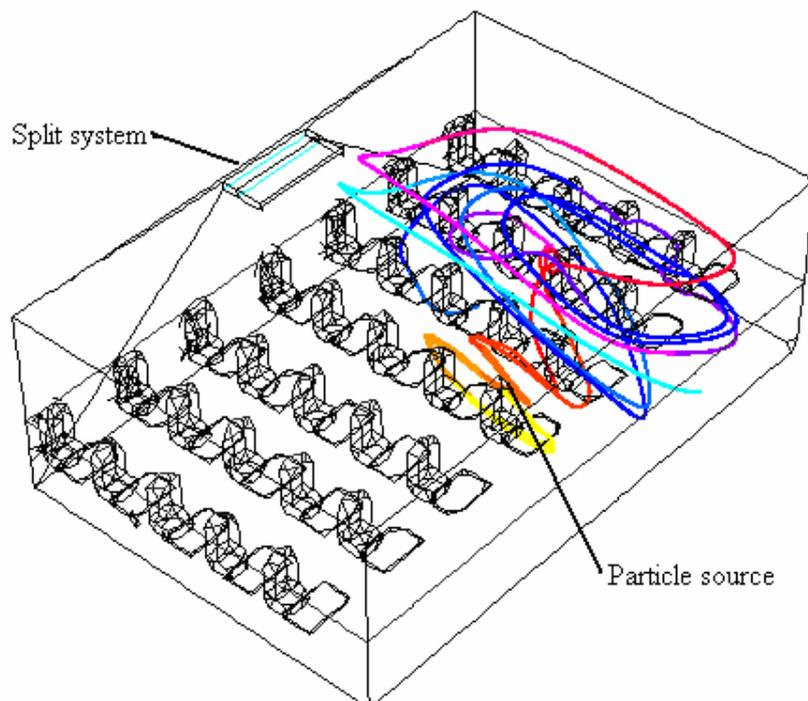
Figure 6. Particle trajectories (1 and 10  $\mu$ m)
