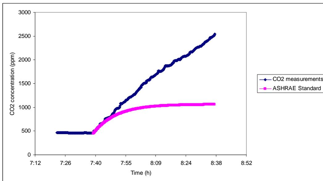
Figure 2. Fluctuation of CO<sub>2</sub> concentration in the classroom compared with AHSRAE recommendation.
