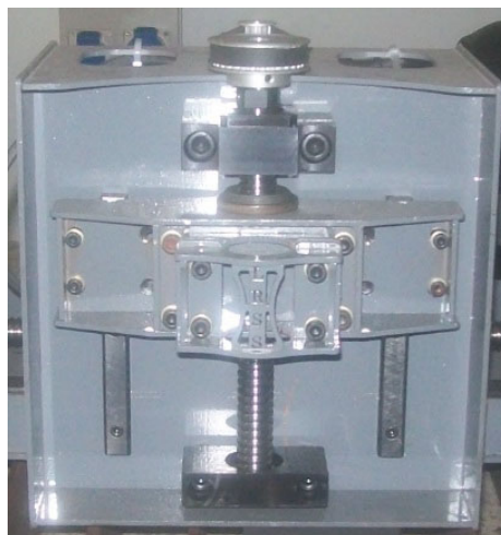
Figure 3 - Application of the LOD method - Support of the plasma cutting torch
