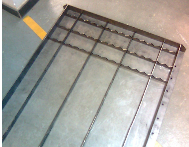
Figure 5 - Fixing of the pallets in the water table
