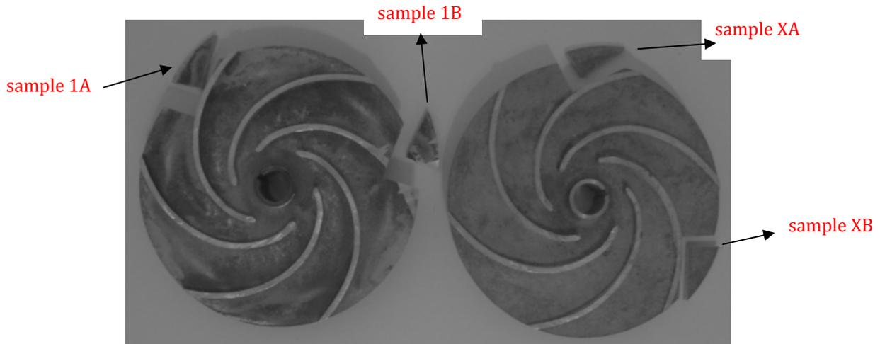
Figure 3. Samples cut from the eroded and new impellers.
