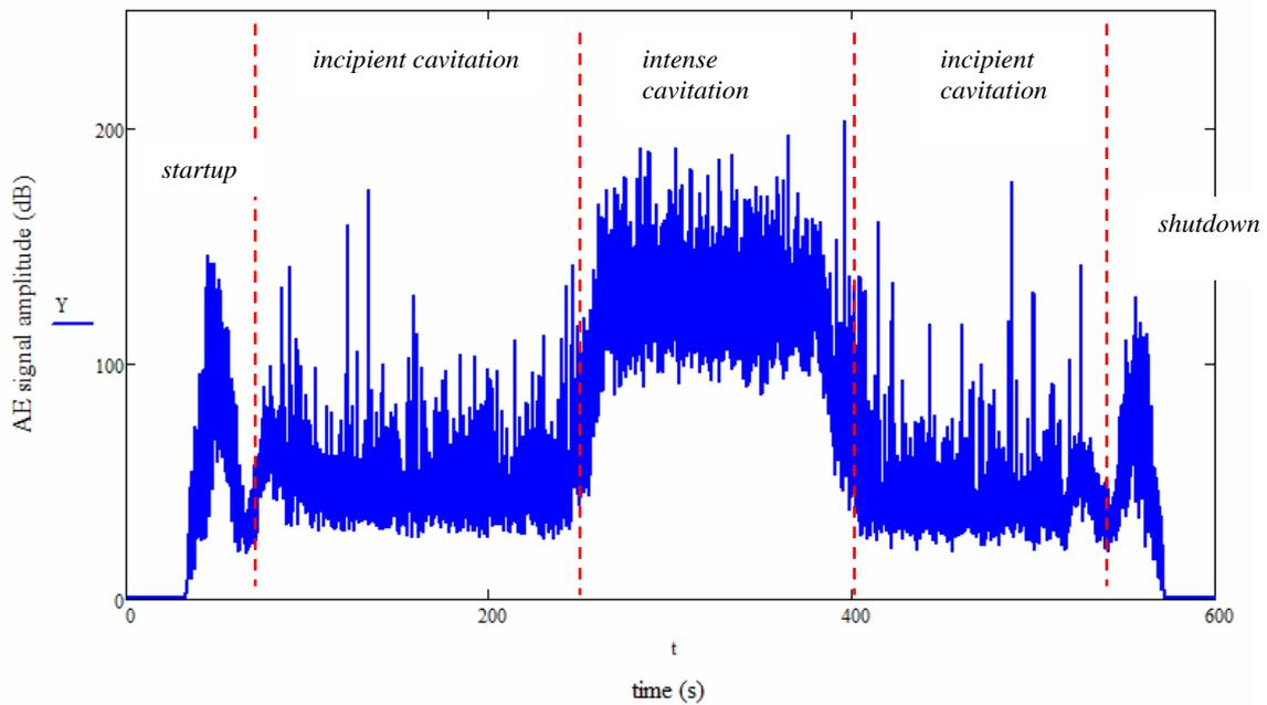
Figure 4. Curve of AE signal amplitude versus time.
