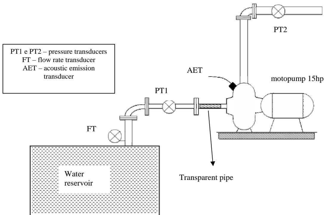
Figure 1. Schematic drawing of the pumping system used in the cavitation tests.
