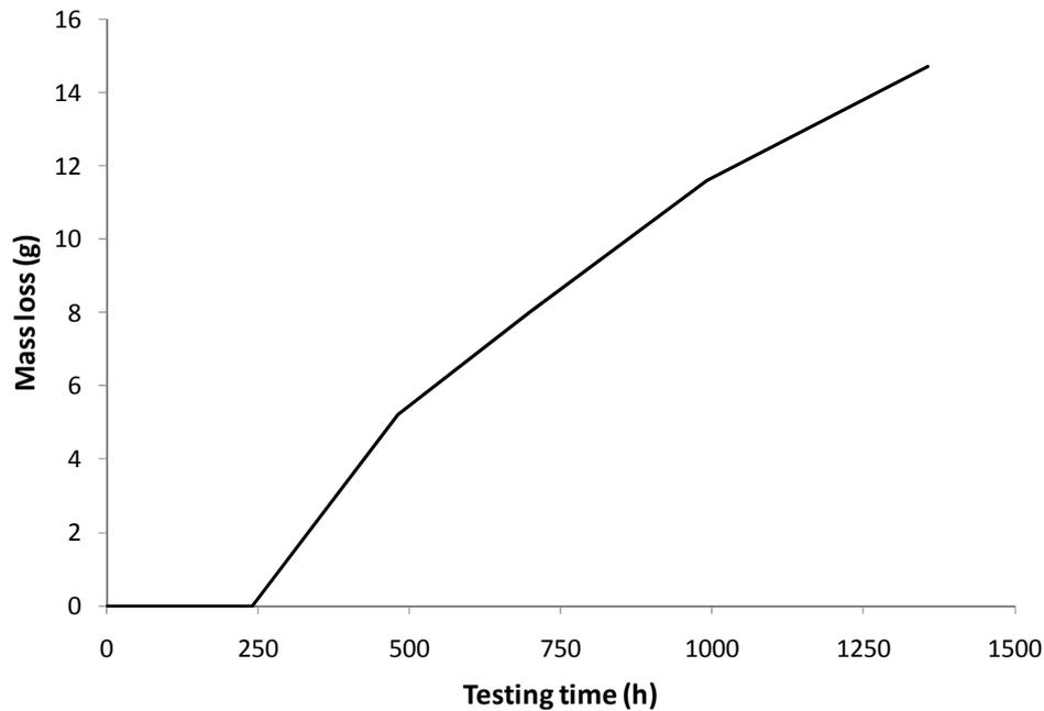
Figure 5. Curve of the brass impeller mass loss.
