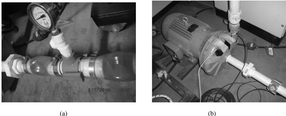
Figure 2. Photographs of the suction pipeline and the motopump: (a) transparent pipe installed at the pump suction line (b) AE transducer mounted on the motopump spiral case.
