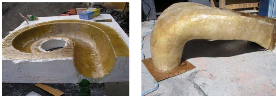
Figure 5. Fiberglass lamination process of the spiral case and draft tube models.
