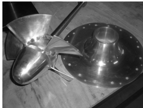
Figure 7. Photographs of the turbine runner mounted on its shaft and of the inlet cone.
