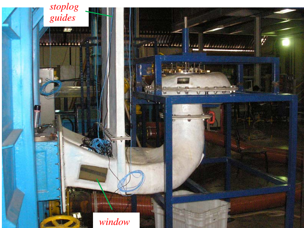
Figure 10. Photograph of the axial turbine model with electromechanical fish barriers.
