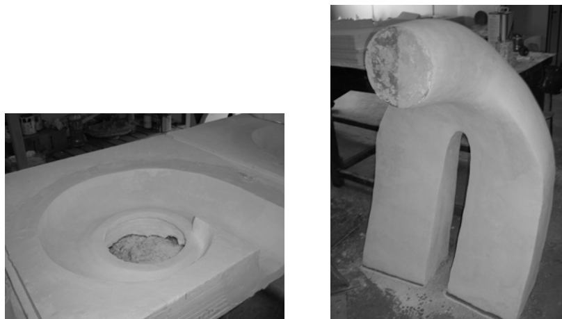
Figure 4. The solid foam models after the geometric rectification by using plaster.
