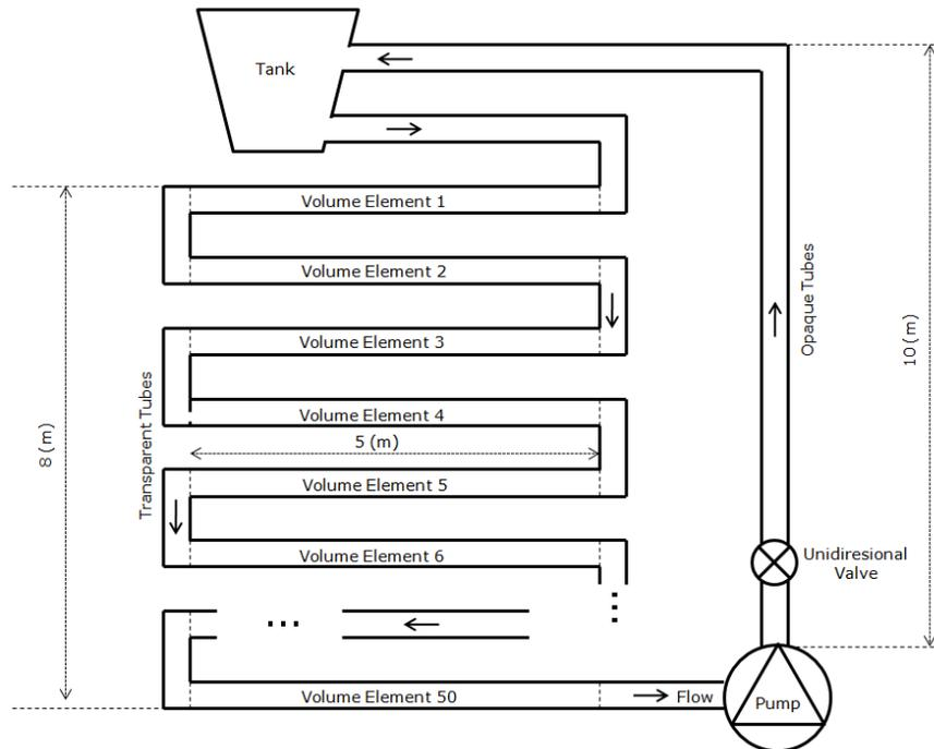
Figure 3 – Simplified schematic of the photobioreactor
