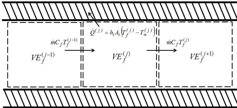
Figure 7 – VE  $j$  for the equation of conservation of energy in the fluid.
