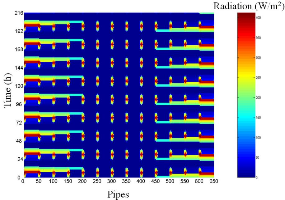
Figure 11 – Visualization of boundary lines of the incident radiation in the tubes of photobioreactor.
