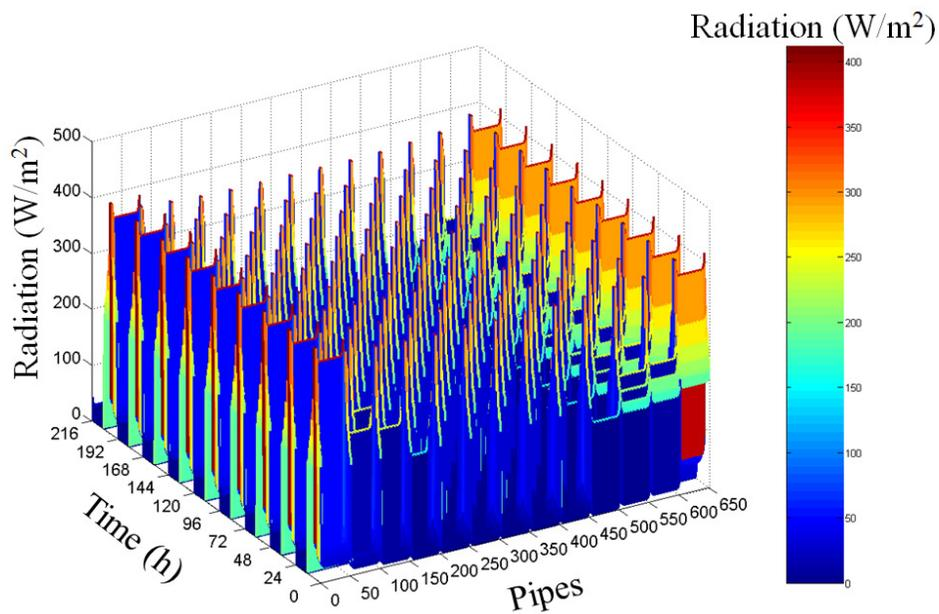
Figure 10 – Incident radiation in the tubes of the photobioreactor during the simulation time.
