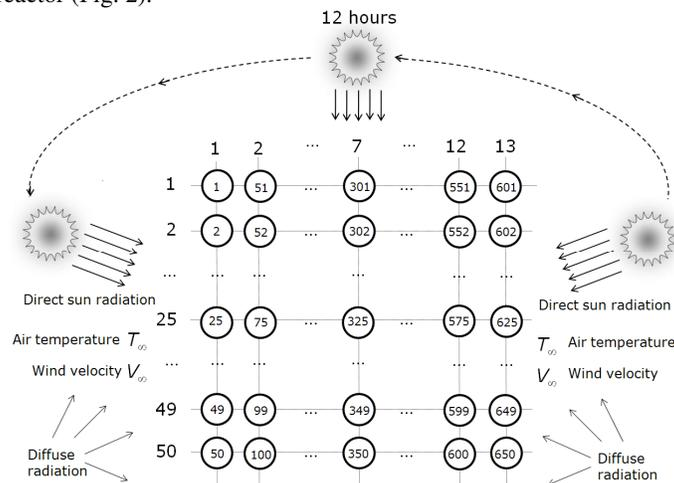
Figure 2 – Photobioreactor geometry and ambient conditions.
