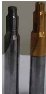
Figure 3 – Cermet carbide drills without and with TiCN coating.
