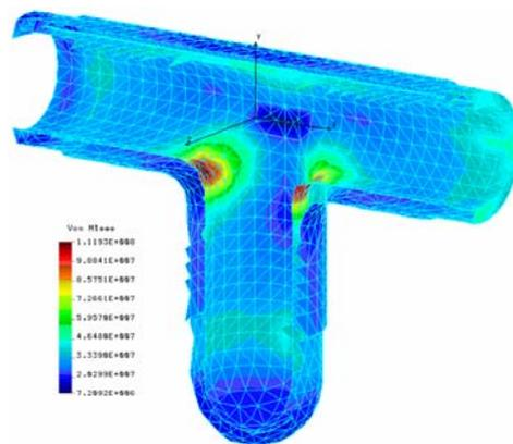
Figure 10. von Mises stress distribution for modified component subjected to 9.8 MPa
