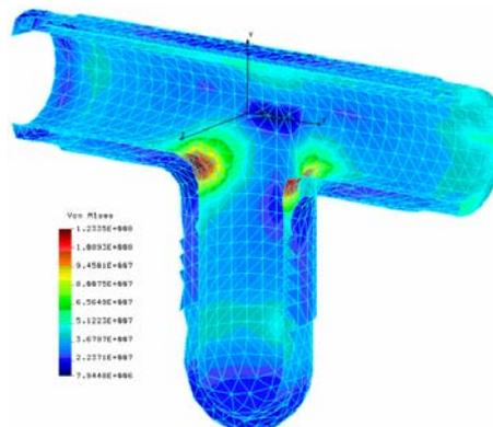
Figure 11. von Mises stress distribution for modified component subjected to 10.8 MPa
