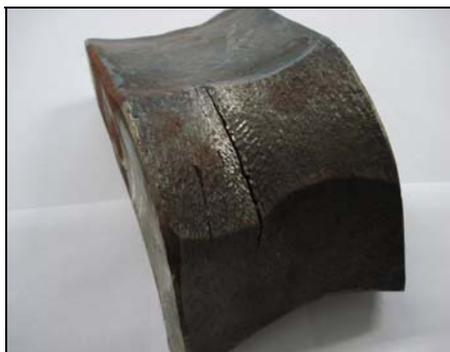
Figure 1. Detail of the internal creep crack in a T-type pipe replaced during maintenance
