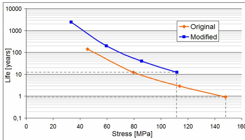
Figure 13. Service life of original model at project condition and modified model at limited operation condition
