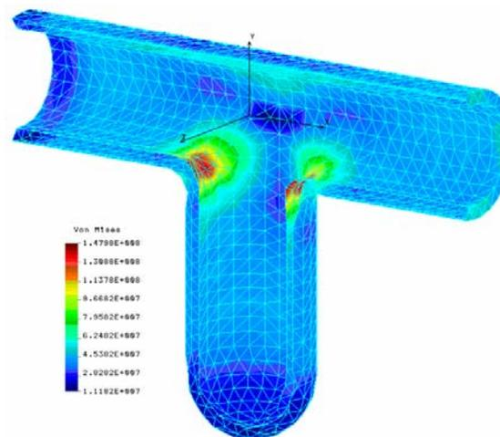
Figure 5. von Mises stress distribution corresponding to project operation condition (10.8 MPa)
