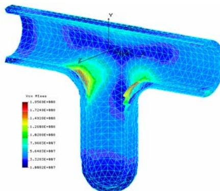
Figure 8. von Mises stress distribution for the first modification proposal subjected to 10.8 MPa
