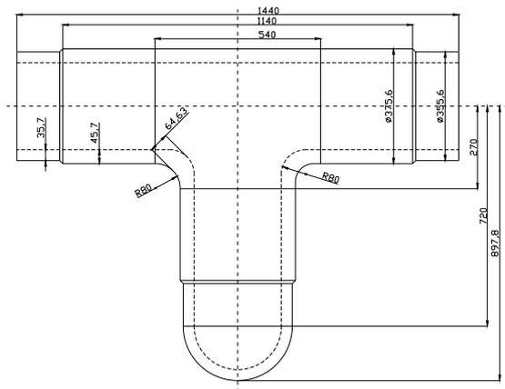
Figure 9. Modification proposal for T-type pipe with nominal diameter of 14 inches
