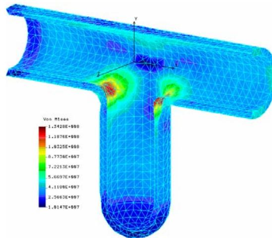
Figure 4. von Mises stress distribution corresponding to limited operation condition (9.8 MPa)
