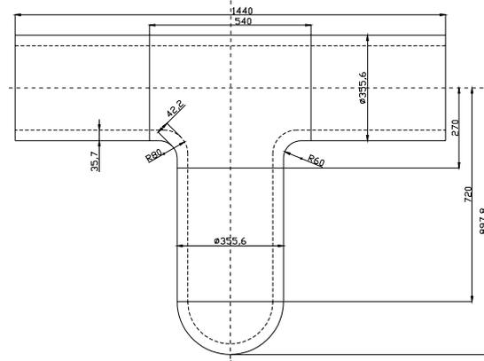
Figure 2. Layout of the 14-inch nominal diameter T-type pipe
