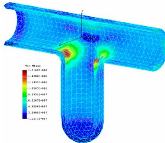
Figure 6. von Mises stress distribution corresponding to extrapolated operation condition (11.8 MPa)
