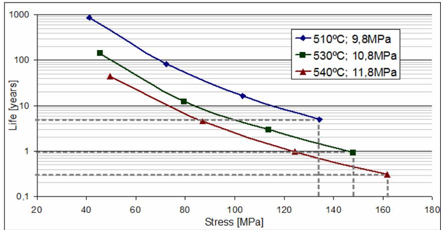
Figure 7. Service lifetime under creep conditions
