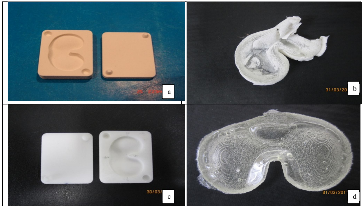
Figure 11 – a- plaster cast; b - PVAI meniscus impregnated with gypsum particles; c - Polyamide Cast; d - PVAI meniscus
