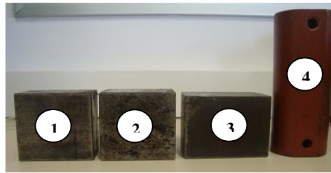
Figure 2. Weights used to stabilize the force on the probe
