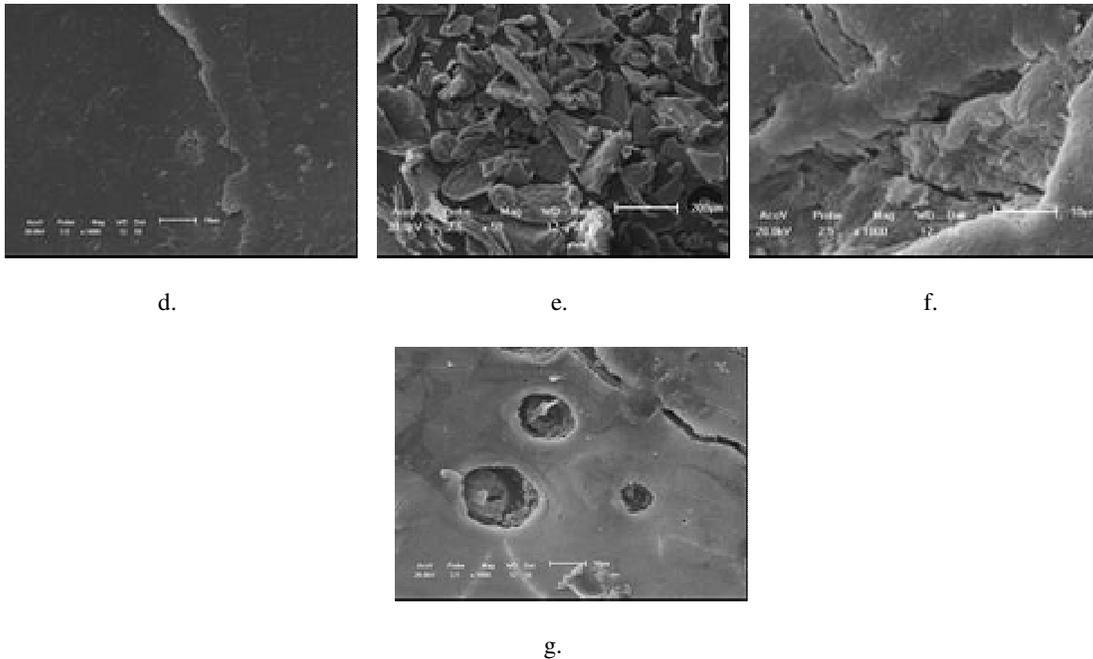
Figure 6. Micrographs of a. Chitin 50 x b. Chitin 1000 x c. Chitin 1000 x d. Chitosan 1000 x e. Chitosan 50 x f. Chitosan 1000 x g. Chitosan 1000 x
