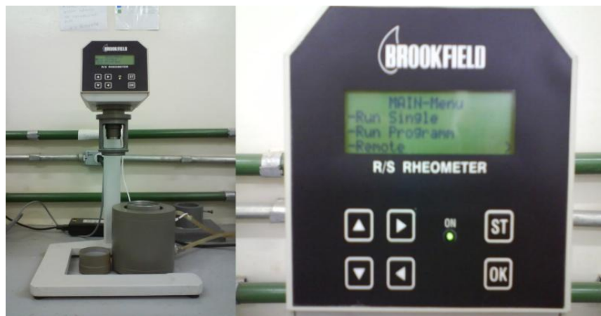
Figure 5. Brookfield R/S Coaxial Geometry Rheometer.
