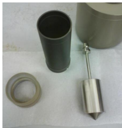
Figure 6. “Spindle” of geometry CC- 45.
