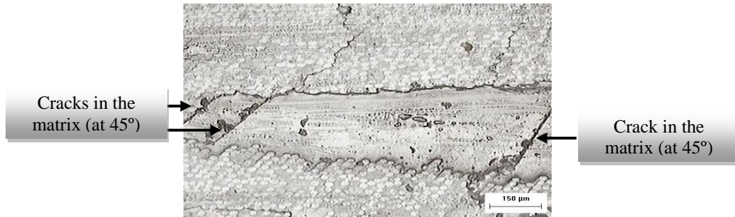
Figure 17. Matrix cracks in the reinforcement direction - HFL ±45° composite.
