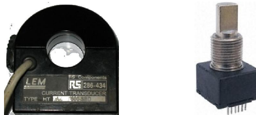
Figure 7- Transducers: LEM HT500-SBD (left) e Bourns EM14 (right).
