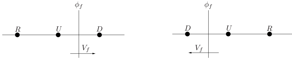
Figure 1. Position of computational nodes D , U and R according to the sign of velocity V_f of a convected variable \phi_f .
