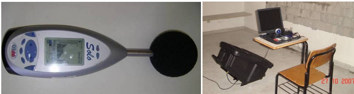
Figure 4: (a) Sound Pressure measurer SOLO SLM 01dB. (b) Loudspeaker model CSR 5500XA and White Noise sound source generator.
