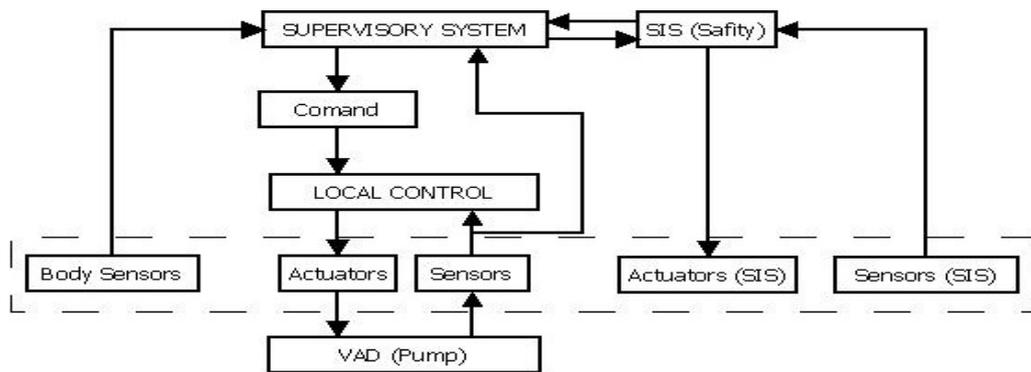
Figure 6 – Control architecture proposed.
