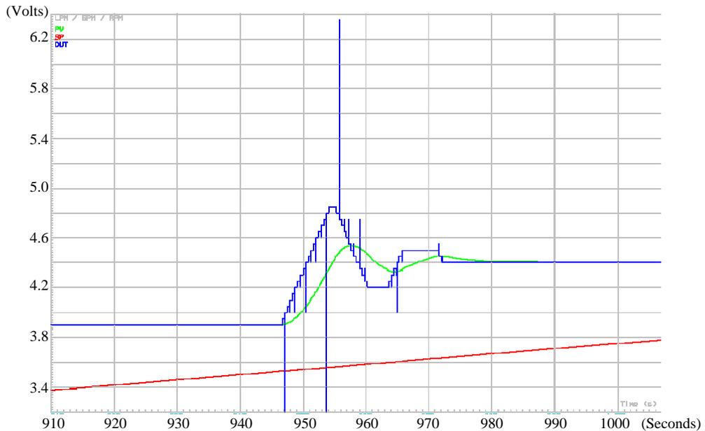
Figure 8 – Pump load changes and reaction of automatic speed control
