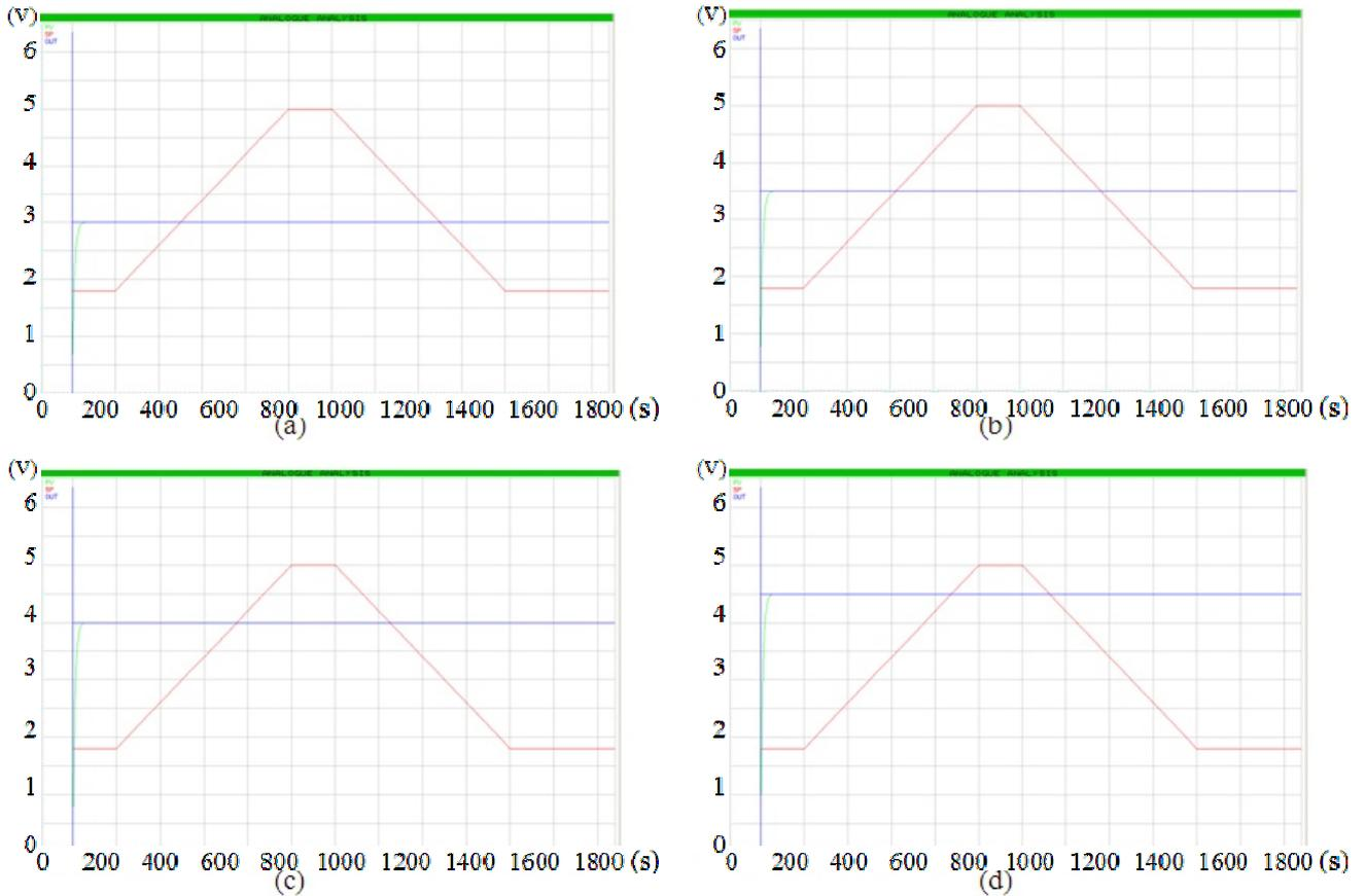
Figure 9 – VAD control system operating in fixed frequency. (a) 100 bpm, (b) 120 bpm, (c) 130 bpm and (d) 140 bpm.
