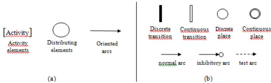
Figure 2 – (a) Production Flow Schema elements; (b) Basic elements of Hybrid Petri Net (Matsuno, 2003)
