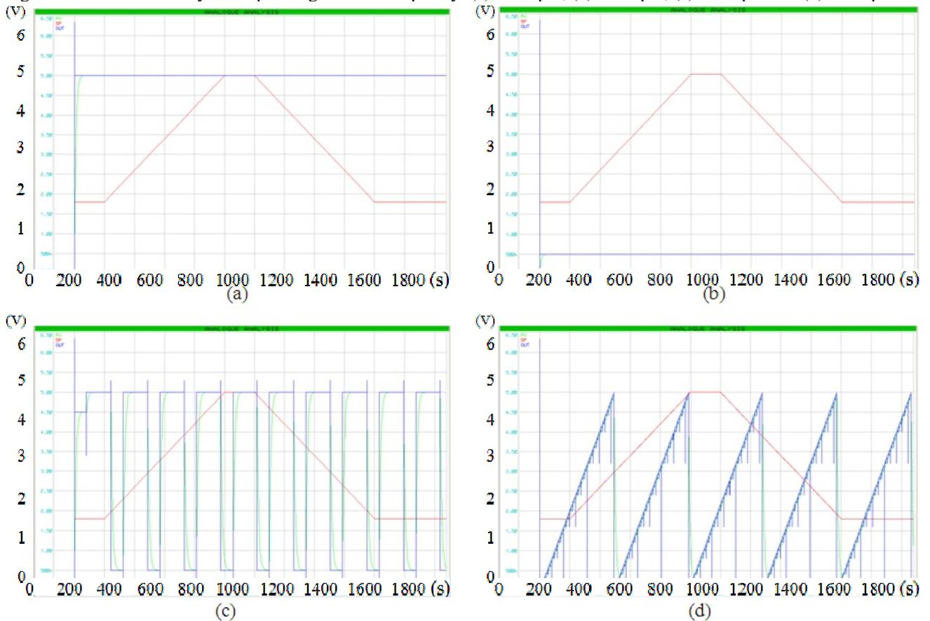
Figure 10 – VAD control system operating in Safety Mode. (a) maximum output speed; (b) minimum output speed; (c) square wave output speed; (d) a triangular wave output speed.
