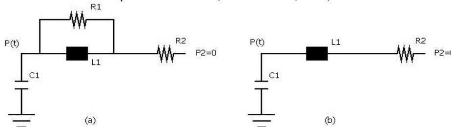
Figure 4 – (a) Electronic elements equivalents arteries with radius less 0.2 cm (b) others arteries.
