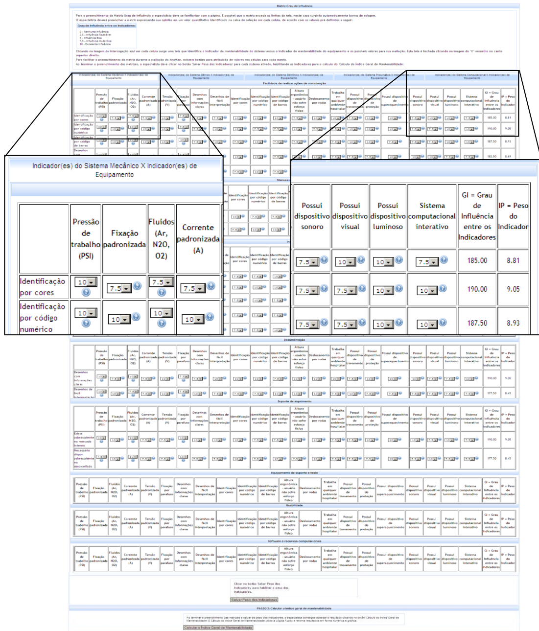
Figure 5. System(s) maintainability indicator Influence degree Matrix - IM_{(SISTEMA)} versus maintainability indicators on the product or equipment function IME_{(EQUIPAMENTO)} (CARMO, 2010)
