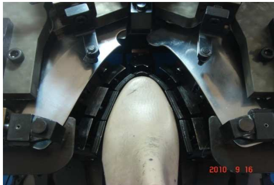
Figure 13 - Contour followed by the pincers around a wide-toed last.
