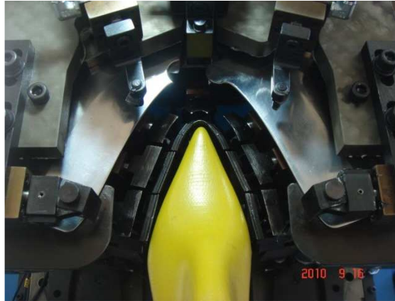
Figure 12 – Contour followed by pincers around a narrow-toed last.
