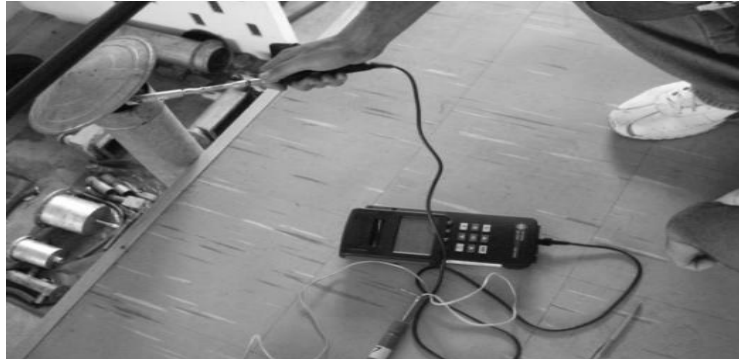
Figure 3. Turbine digital anemometer acquiring velocity data and gas temperature.
