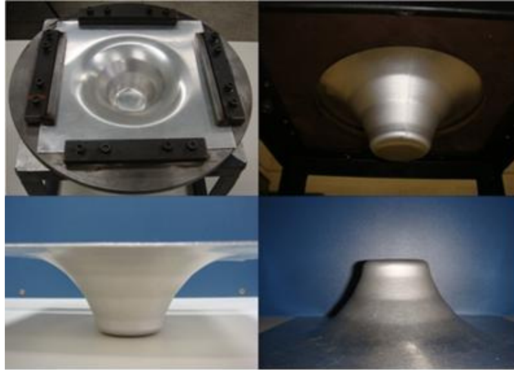
Figure 10. Cone with constant work angle, obtained by SPIF.
