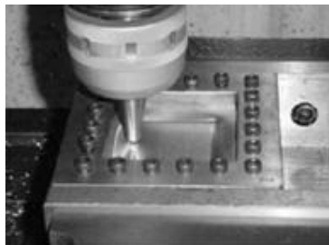
Figure 1. Single Point Incremental Forming process (Dieless, Negative and Symmetrical)
