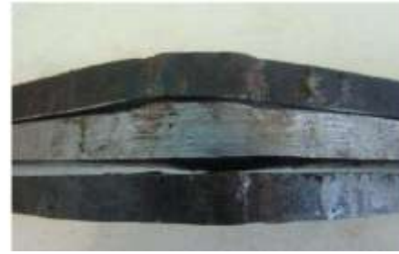
Figure 12. Bend Test, FCAW-S, wind speed of 4.4 m/s
