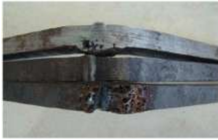
Figure 11. Bend Test, FCAW-G, wind speed of 2.3 m/s
