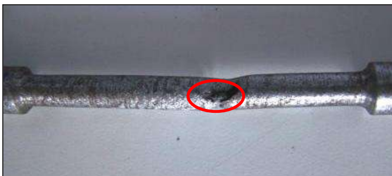
Figure 26. Brittle Slag Inclusion FCAW-S - Winds of 2.3 m/s.
