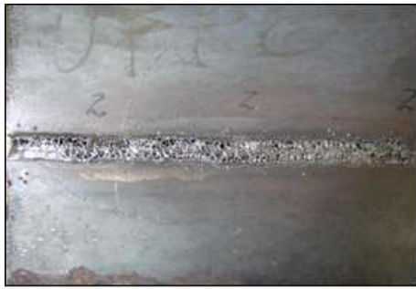
Figure 5. FCAW-G; wind speed of 2.3 m/s Figure 6. FCAW-G; wind speed of 4.4 m/s
