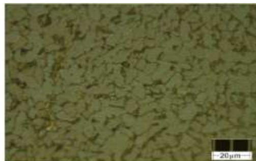
Figure 21. HAZ, FCAW-S, winds 4.4 m/s (Magnification 1000x)
