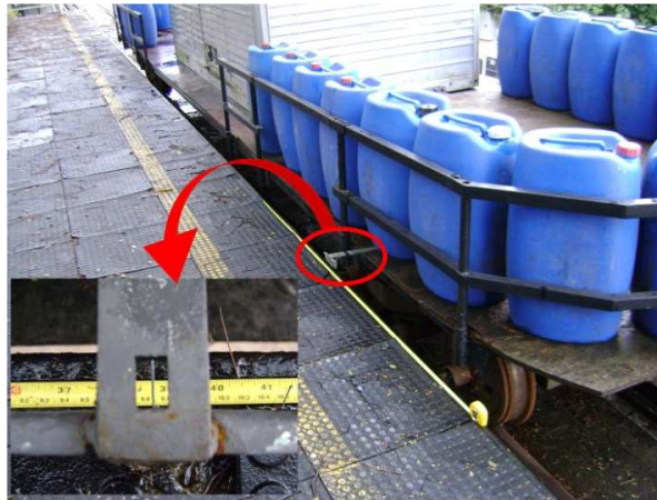
Figure 8. Method to measure the brake error.
