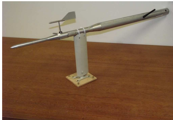
Figure 4. Final aspect of the Pitot tube
