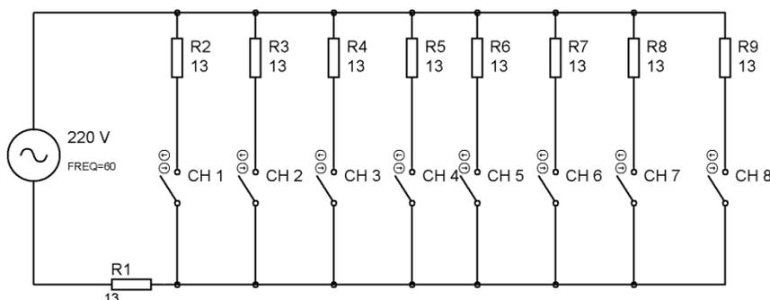
Figure 1. Resistive circuit used to dissipate the electrical power generated
