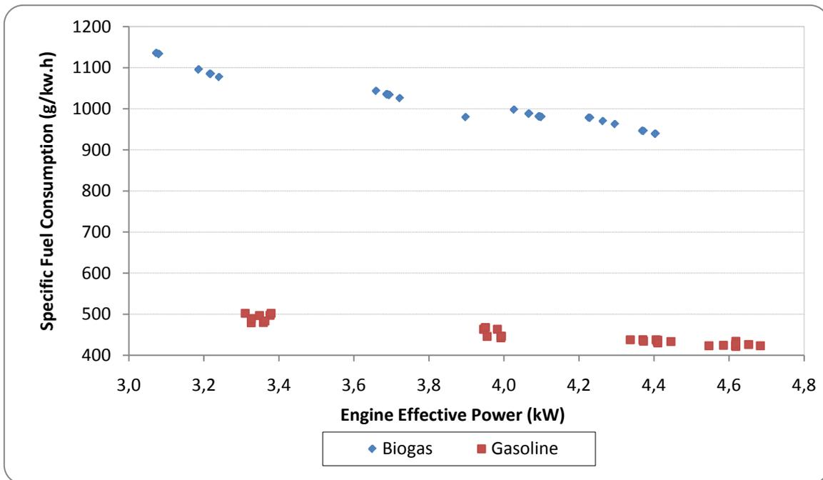
Figure 6. Comparative graphic Engine Effective Power X Specific Fuel Consumption
