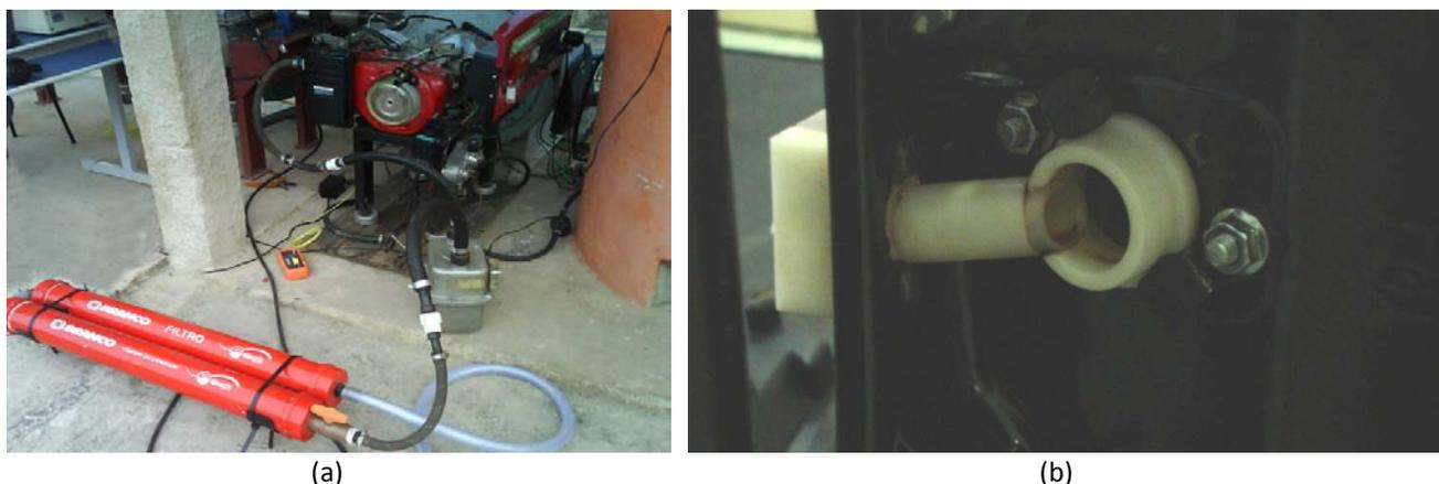
Figure 2.  $\text{H}_2\text{S}$  and balancing chamber (a) and gas diffuser at the engine admission (b)
