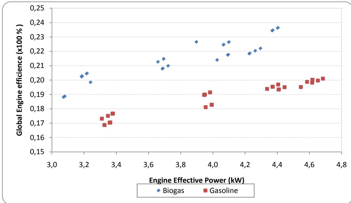
Figure 4. Comparative graphic Engine Effective Power X Global engine Efficiency
