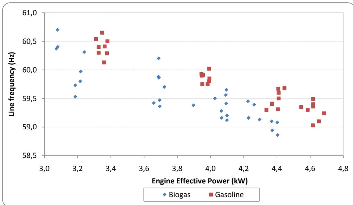
Figure 8. Comparative graphic Engine Effective Power X Line Frequency
