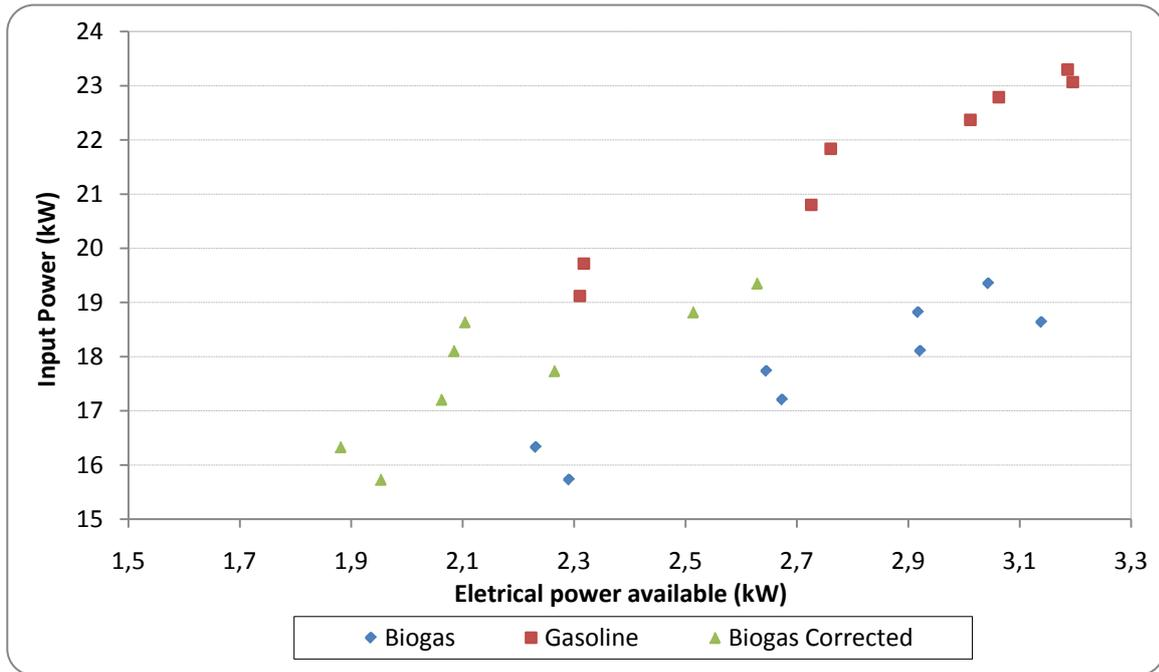
Figure 5. Comparative graphic Electrical Power Available X Power Input
