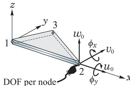
Figure 1. Degrees of freedom of the triangular plate element.
