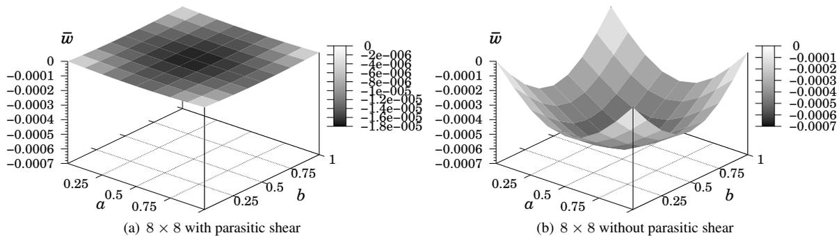
Figure 3. Non-dimensionalized transverse displacement,  $\bar{w}$ , at the center of the plate for side-to-thickness ratio  $a/h = 100$ :  $8 \times 8$  mesh.
