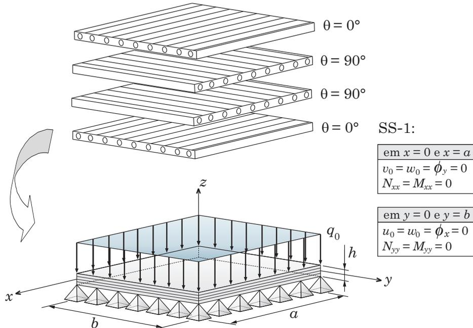
Figure 4. Geometry, lamination scheme and boudary conditions of case 2.
