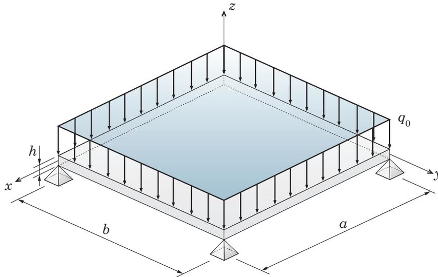
Figure 2. Geometry and boudary conditions of case 1.
