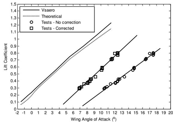
Figure 6. ACS-Sora Lift Coefficient Curve.
