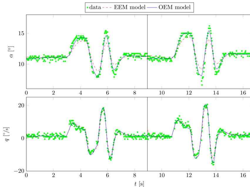
Figure 5. Output of the short-period models against the data used for estimation.
