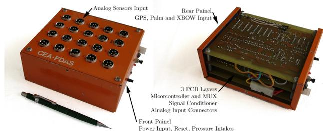
Figure 4. Final Hardware Assembly of the CEA-FDAS.
