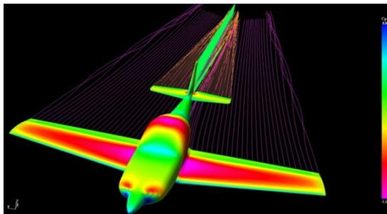
Figure 8. Snapshot of the Output Generated by VSAERO
