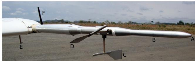
Figure 7. Flow Direction Indicator and Pitot Tube Used During the Flight Tests Campaign.
