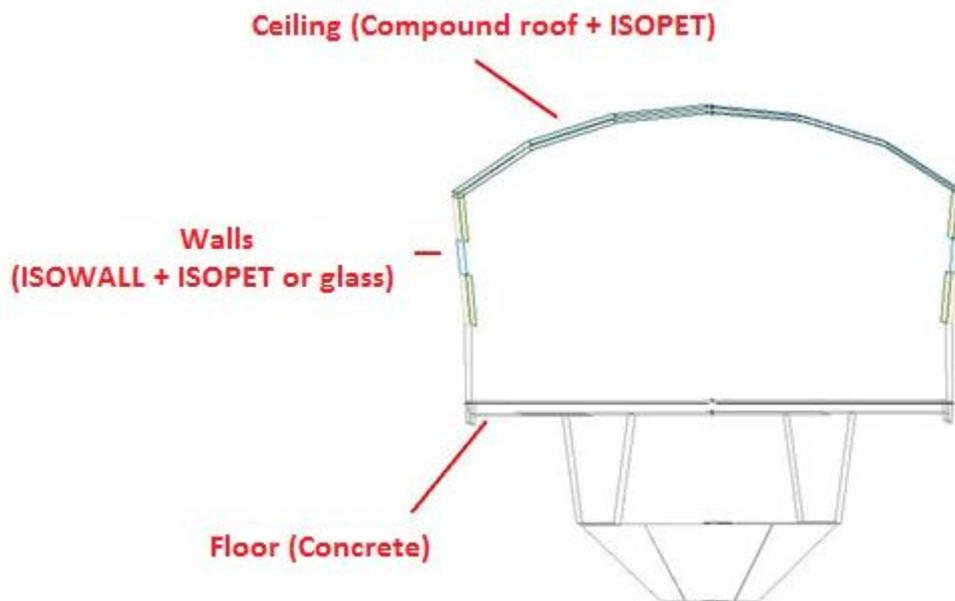
Figure 1. Cross section of the subway line with the acoustic barriers installed.
