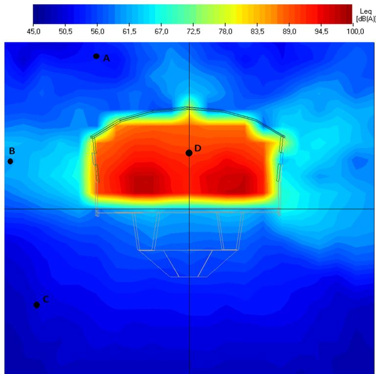
Figure 3. SPL simulated on the computational program considering the situation of two subway trains crossing at a speed of 100 Km/h in the acoustic closing section.
