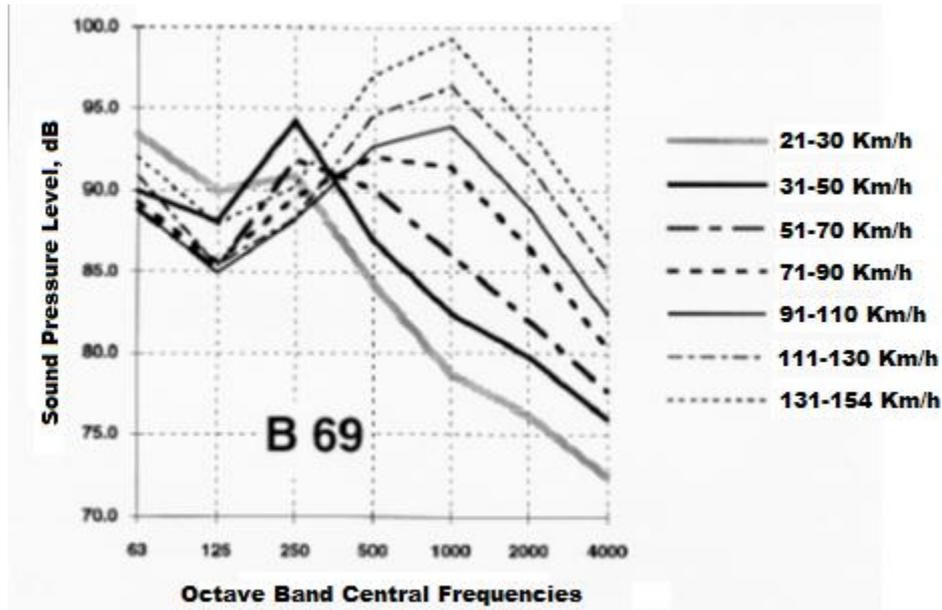
Figure 2. Frequency spectrum used for the estimation of the SWL values of the subway for simulations and calculations.
