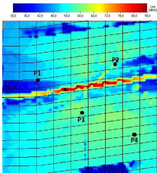
Figure 6. Sound Pressure Isocurves of the simulated subway stretch.
